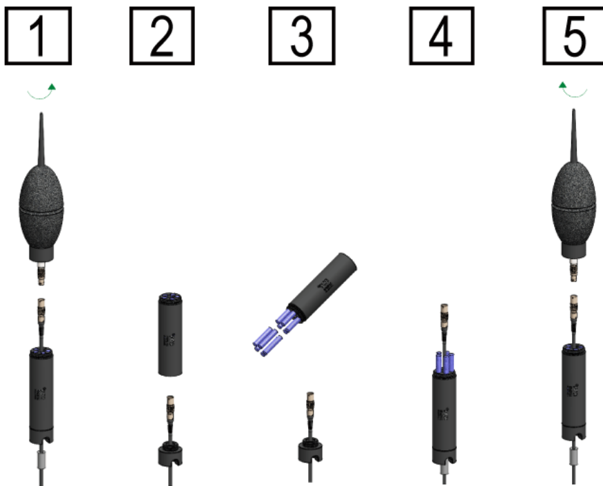
FIGURE 3-3 Replacing EPS2116 Desiccant Cartridge
